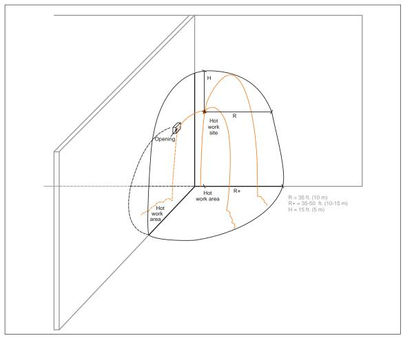
Fig. 5. Elevated hot work permit-required area
