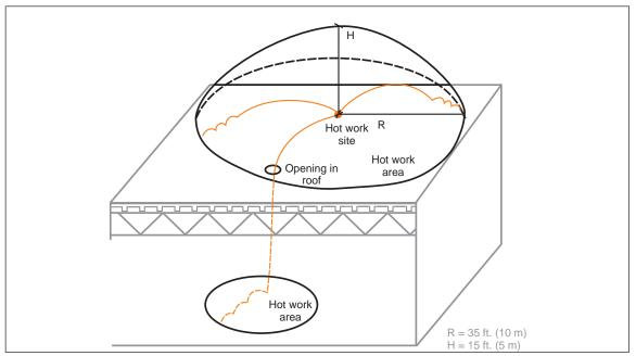
Fig. 4. Rooftop hot work permit-required area
