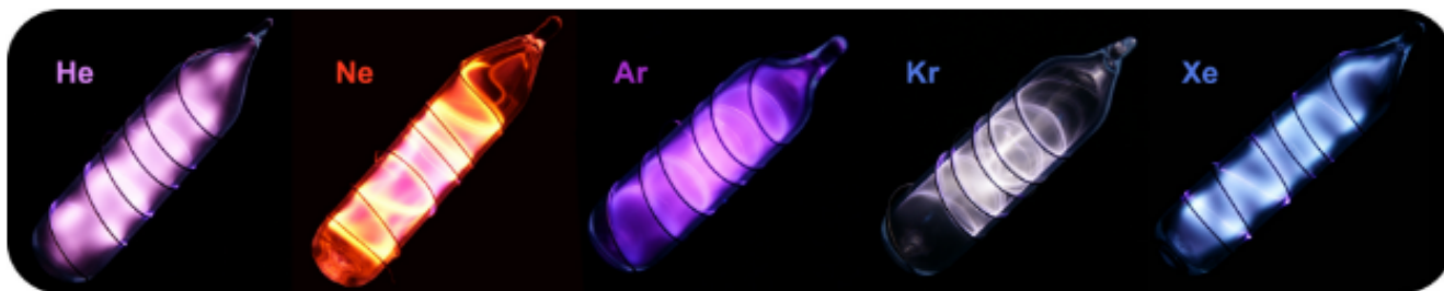
Figure 13.3: Gas discharge tubes are enclosed glass tubes filled with a gas at low pressure through which an electric current is passed. Electrons in the gaseous atoms first become excited, and then fall back to lower energy levels, emitting light of a distinctive color in the process. Shown are gas discharge tubes of helium, neon, argon, krypton, and xenon.
