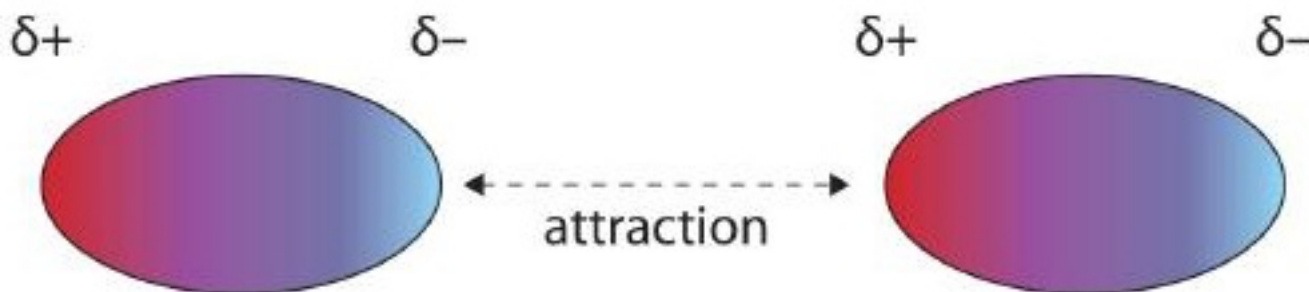
Figure 10.1: Dipole-Dipole Interactions - Oppositely charged ends of polar molecules attract each other.
