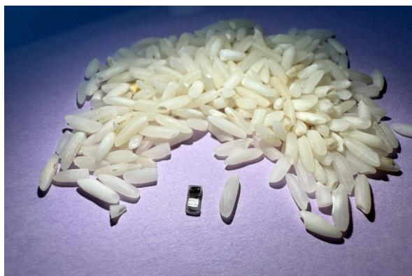
Northwestern engineers developed a pacemaker smaller than a single grain of rice, particularly suited to the tiny hearts of newborn babies with congenital heart defects. Designed for those who only need temporary pacing, the pacemaker dissolves after it is no longer needed. Its components are biocompatible and naturally dissolve in the body's biofluids, avoiding the need for surgical extraction.
