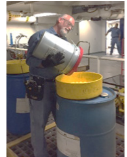
Dave St. Aubin, Engineer, using a spill kit funnel over a containment to prevent a chemical spill
