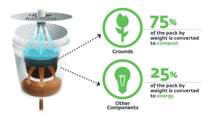
Specifically, the K–Cup pack is processed through a grinding and separation -method that ultimately separates the coffee and tea grounds from the other K–Cup pack components. The grounds are sent out for composting to be used in a variety of agricultural applications, while the remaining K-Cup pack grinds are provided to Covanta Energy and are used in an energy-from-waste process. To learn more about this recycling program, please visit <u>Grounds to Grow On</u>.
