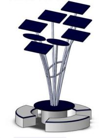
The current design is an 18-foot aluminum structure which resembles the shape of a tree. The 'branches' of
