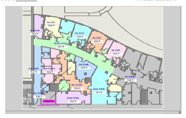
Figure 4: Detailed Floor Plan Graphic Example
