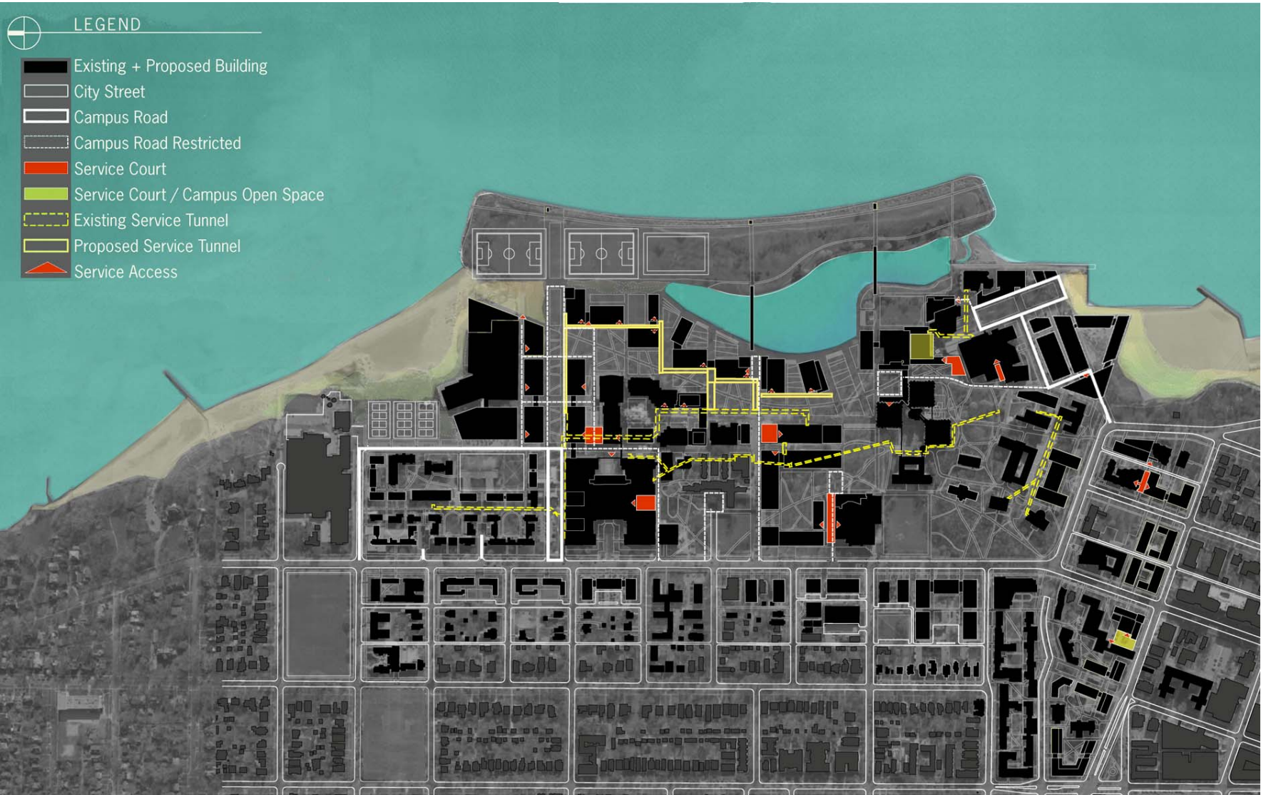
Existing and proposed service and emergency access
